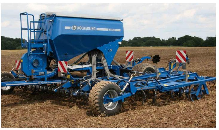
This image shows a JOCKEY 600 pulled by a Valtra 140 hp on a farm near Newbury. The land was cultivated once after OSR. When it comes to light land, the front-Levelboard mounted across the machine helps to eradicate tracks and to level the land. This allows for precise seed-placement even at high speed.
